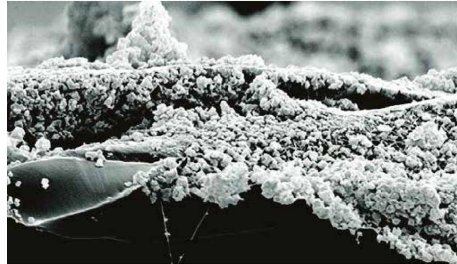
Nanofibre media is loaded with ISO fine dust. Dust particles collect on the surface of the media and vibrate off with equipment use – allowing the filter to last longer.
