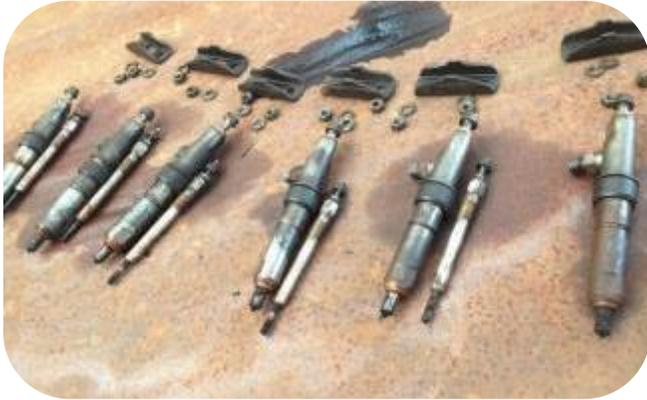
Damaged fuel injector
