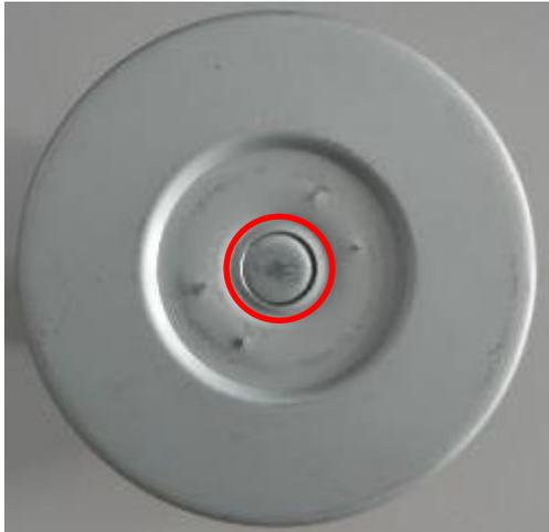
No seal, dirt particles pass the engine
