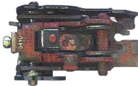
Parts corroded by water contaminated fuel
