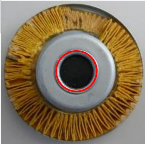
Delay in oil pressure build up on starting
