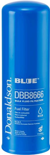
Donaldson DBB8666 contains D.E.R.T. (Donaldson Electrostatic Reduction Technology) to minimise the known effects of Electrostatic Discharge at high flow rates, ensuring your bulk fuel filtration provides the targeted ISO Cleanliness of 14/13/11 for the duration of its service life.
