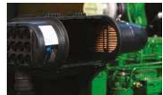
The safety filter should be replaced every three primary filter changes.
